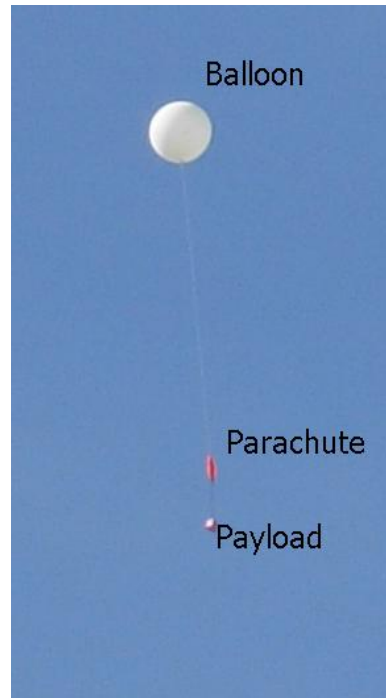
Figure 3 - High altitude balloon configuration.
