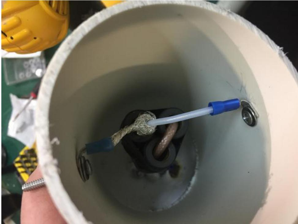
*Figure 1: The balun after rebuilding*
