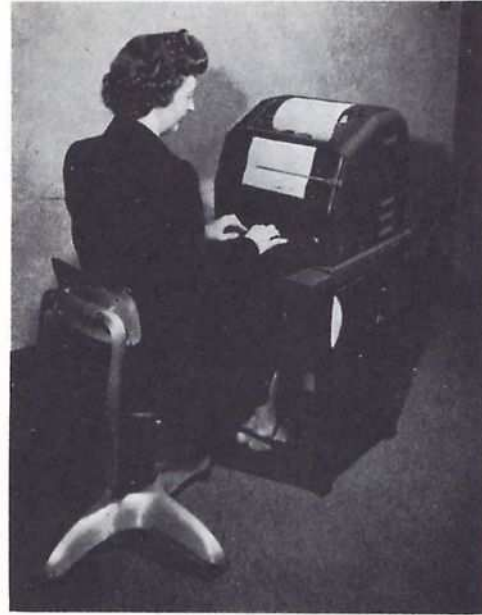
Fig. 12-4. The teletype is an important device used today to send messages. It has replaced the former Morse Code method of sending messages.
