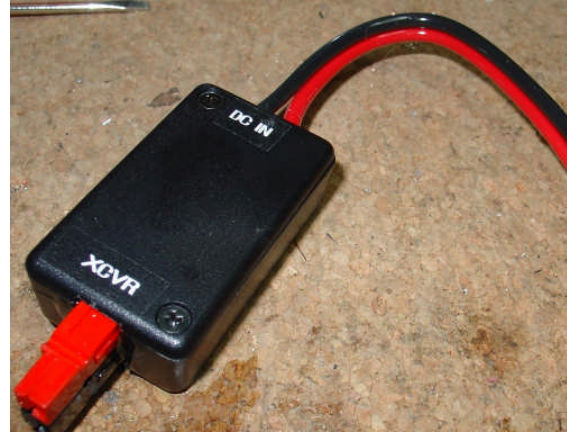
Photo D: Final cartridge fuse assembly
