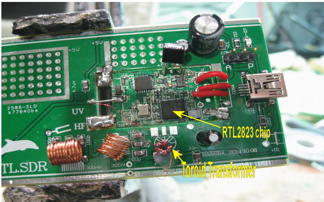
Not to imply that there are instructions to tell you to do this, but to get the HF side to work, pins 4 and 5 of the RTL2823 chip need to be soldered directly to the balun/toroid transformer secondary side. These pins represent the Q-/Q+ signal inputs and are unused on the stock board. I got the best results by using a 4:1 ratio and not grounding the centre tap on the secondary, but YMMV.
