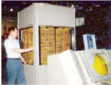
Major Dave Lawrence stands beside 4 Kilobytes of 32 Bit memory from a 1962 Mainframe. If it weren't for microchip technology, it would take 2,000 of these units to run Microsoft Windows. (Courtesy: C & E Museum)
