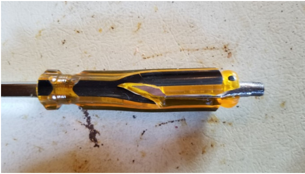
Screwdriver showing split handle and threads.
