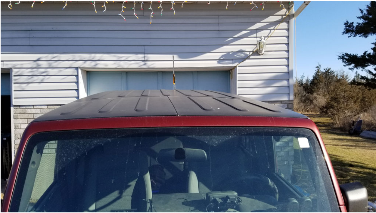
2m Screwdriver antenna from front of Jeep, radio control head and speakers can be seen on the dash
