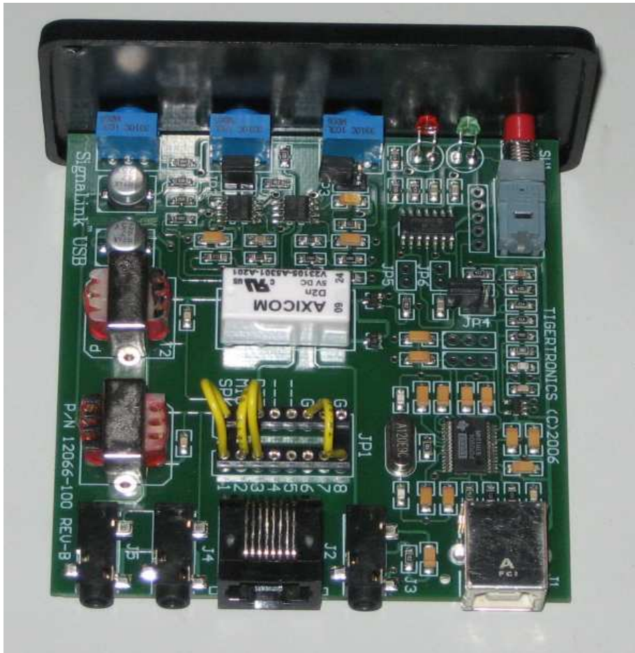
Figure 1: Yellow jumper wires (included) configure the unit to operate with the IC-7000 in this case. Notable features are high-quality SMD construction and audio isolation transformers. The 3 extra jumpers (JP2, JP3, and JP4) are there to help expand the unit's compatibility to work with virtually any radio.
