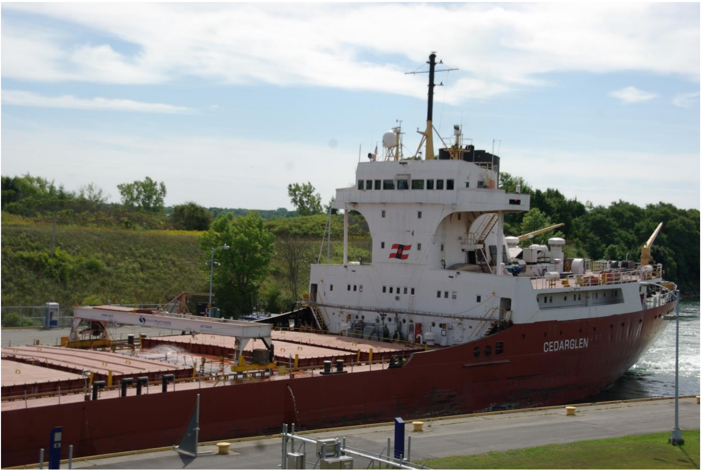
6 The metal above water gets hot and the metal below water stays cold. Thus the top expands and the ship bends so the bow and stern go deeper than allowed. Decks are cooled so the ship stays on an even keel.
